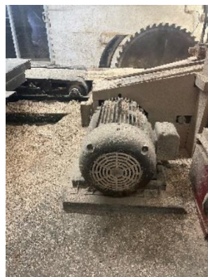
Electric motor Baldor 100 Hp Log saw 52 inch
