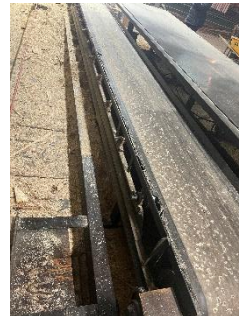
Strap conveyor 2 x 20 feet with 3 Hp motor
